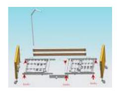
Install the side panels and secure the frame with the locking clamps, pulling outwards as shown in the next image.
