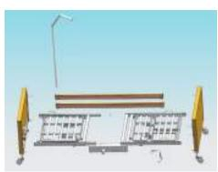
Assemble the two parts of the bed and secure them using the 4 screw knobs contained in the product package.
