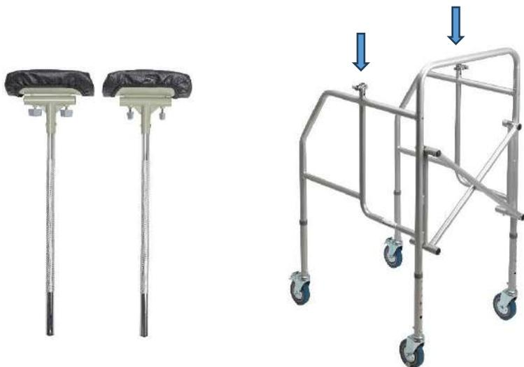
You can adjust the height of the armpit supports with an upward or downward movement. After choosing the desired height, close the locking lever in the knurled area on the armpit supports.
