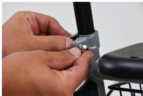
6) Check that the screw is fully inserted, making sure that the protruding stop in the head of the screw fits into the groove.
