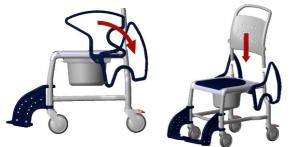
3. Swivel the armrests forwards until they click into the slots of the backrest and the locking pins click into the lower frame. Be sure they are securely in place.
