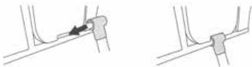
C. Insert four legs into the holes below the bath seat, then assembly completed;
