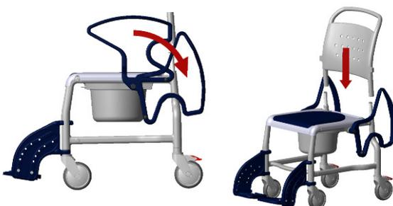
3. Swivel the armrests forwards until they click into the slots of the backrest and the locking pins click into the lower frame. Be sure they are securely in place.
