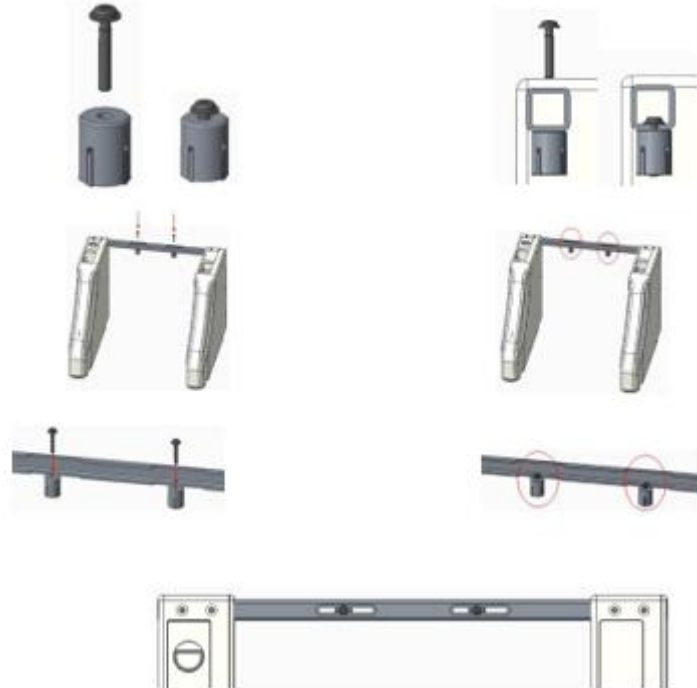
Figure 7.1 : The equipment is attached to the toilet with bolts
